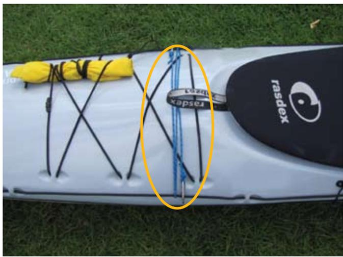
Left: The bungee tow on the deck lines, Above: The Short tow stowed, Right: The dog leash, Below: The bungee direct tow - note Steve is able to hold onto the rear of James' kayak.
